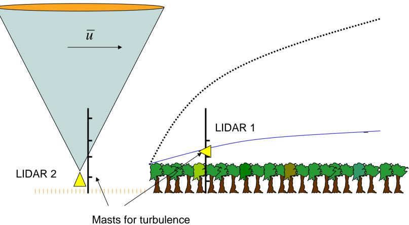
and mean wind speed measurements
