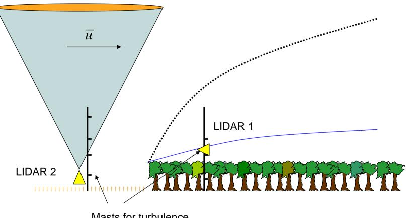
Masts for turbulence and mean wind speed measurements
